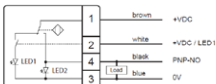
Connection diagram „P“ PNP-NO // Semi-Automatic
