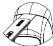
Removal of the HWT2 cup Special tool „HWT2-DW“
